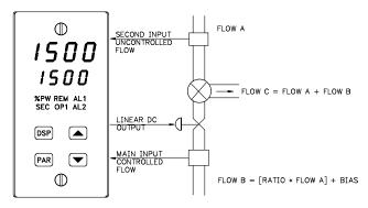
The PCU configured for ratio operation controls a process as a ratio of another process or to another variable. Ratio control is commonly used for flow applications, however, any two process variables can be controlled in a ratio mode.
