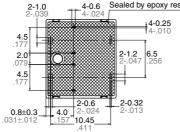
Dimension: Tolerance Max. 1mm .039 inch: ±0.1 ±.004 1 to 3mm .039 to .118 inch: ±0.2 ±.008 Min. 3mm .118 inch: ±0.3 ±.012
