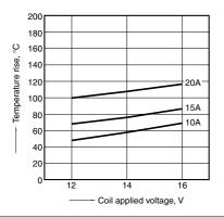
1-(5). Coil temperature rise (at room temperature) Sample: ACJ5212, 3pcs Measured portion: Inside the coil Contact carrying current: 10A, 15A, 20A
