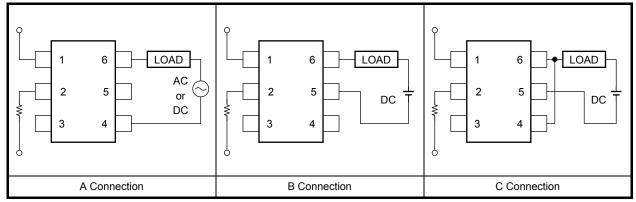
Note 1: Device considered a two-terminal device: LED side pins shorted together, and DETECTOR side pins and 6 shorted together.
